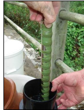
Fig. 14 Fine sediment retained on magnet
