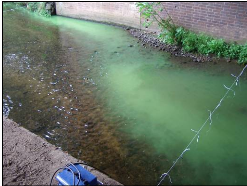
Fig. 13 Sediment tracer at 40.0 m downstream from outfall
