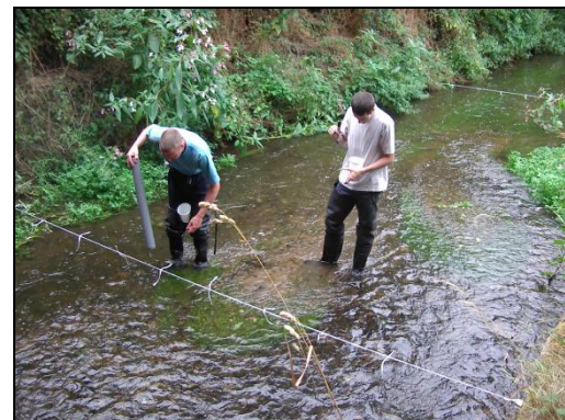
Fig. 10 Discrete bed core samples taken at 0.5m intervals
