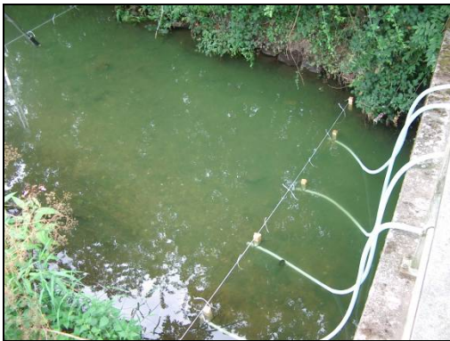
Fig. 7 Suspended sediment sample extraction
